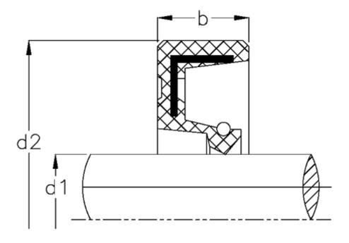
$\begin{array}{ll} b & = 12 \\ d1 & = 80 \\ d2 & = 110 \\ Material = NBR \end{array}$
